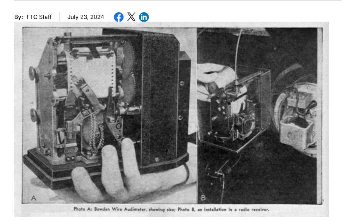
This photo from a 1945 issue of Radio-Craft magazine shows the inside of a radio Audimeter, a device used to monitor what households were listening to on their radios. This picture gives us a rare peek inside one of the first "black boxes" that collected consumer data. <u>Source</u>
