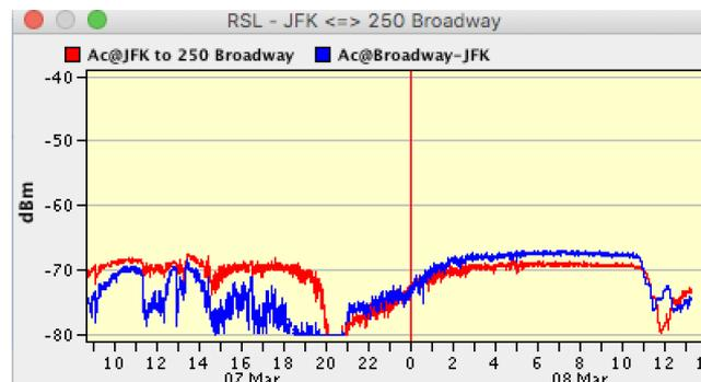
When the receive levels drop below about -75 dBm, this microwave link cannot maintain a data channel. As you can see, there's not much margin
