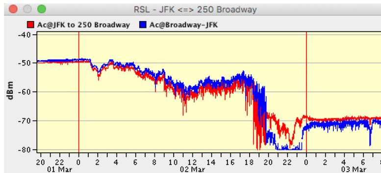
As a result, this link was more adversely affected by snow buildup last night than other similar links. At the -70 dBm receive levels shown on the right of the chart, this link is operating on the edge, and is barely able to maintain a viable data link.
