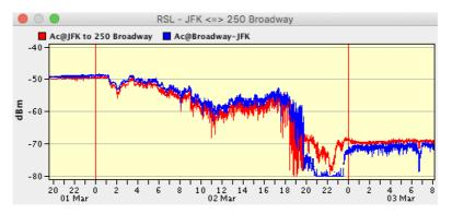
As a result, this link was more adversely affected by snow buildup last night than other similar links. At the -70 dBm receive levels shown on the right of the chart, this link is operating on the edge, and is barely able to maintain a viable data link.
