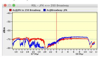
When the receive levels drop below about -75 dBm, this microwave link cannot maintain a data channel. As you can see, there's not much margin
